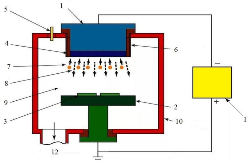
Figure 1 – A schematic of the PVD coating process:
