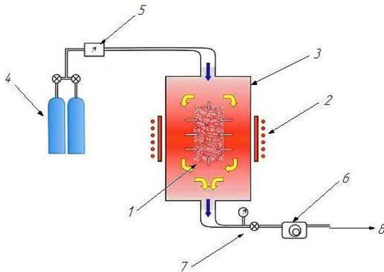
Figure 2 – A schematic of the CVD coating process:
