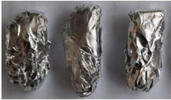
Figure-1. LiF wrapped in aluminum foil.
